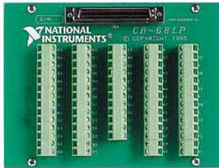
Abb. 2.4.3: Data Acquisition-Board NI CB-68LP (National Instruments Germany GmbH, 2013)
